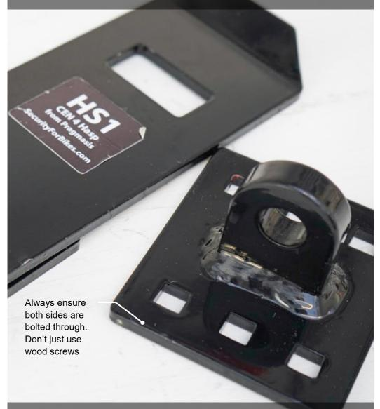
Quality hasp sets have a vertical staple eye. This allows a closed shackle padlock to hang properly. A horizontal eye means a closed shackle lock will protrude outwards making it more vulnerable to attack with a hammer.
